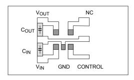
Board material: Glass Epoxy, Board dimension 30 mm  $\times$  30 mm
